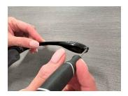
1. Using a small Phillips screwdriver, unscrew the 2 screws in the end of the glasses arm with the On/Off switch.
